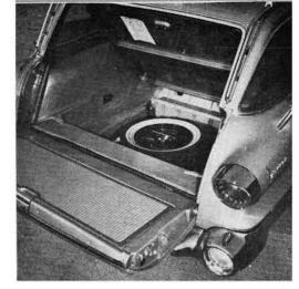
TAILGATE is quite wide and well designed for loading. Only drawback is fact that it does not lie flat with floor due to rubber bumper guards.
