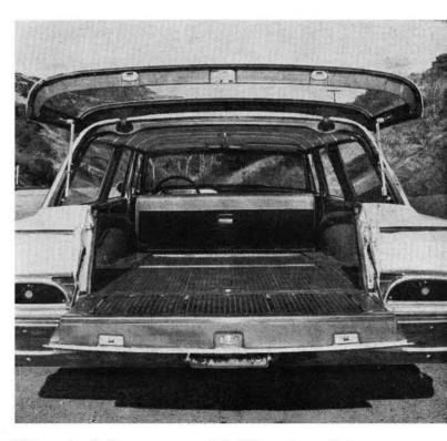
FORD remains the lone proponent of the lifting tailgate window. Its 61.1-inch width has loading advantages but they are offset by an extremely narrow down-swinging tailgate. On nine-passenger versions, rear seat faces front instead of to the rear.
