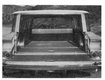
LOADING the Chevy wagon is hindered by a tailgate opening which is 20 inches narrower than the cargo compartment itself. Spare and tools are stored beneath small door located behind the tailgate.
