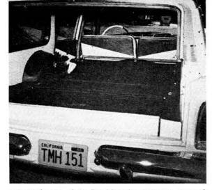
UNIQUE feature of the Rambler nine-passenger wagon is a full-swinging door at the rear rather than normal tailgate. It has a big advantage in access to loading area and the rear passengers don't step over a gate.
