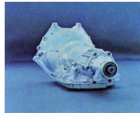
3-speed Turbo Hydra-Matic. Extra-cost, any engine. You can get a 400 cu. in. 255-hp 2-bbl with it.
