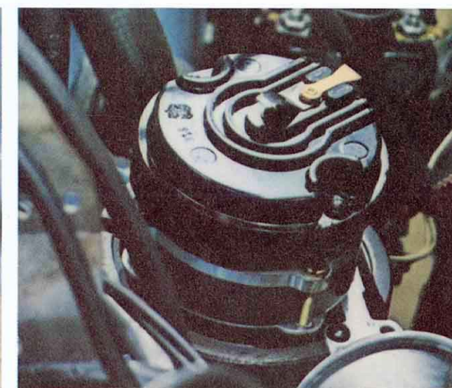
Delco transistorized ignition. It's the next best thing to a magneto. Extra cost.
