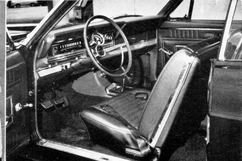
Fairlane's interior is identical to any GT job with the exception of 9-grand tach mounted to right of steering wheel. Though not available yet, C6 Ford-O-Matic is coming.
