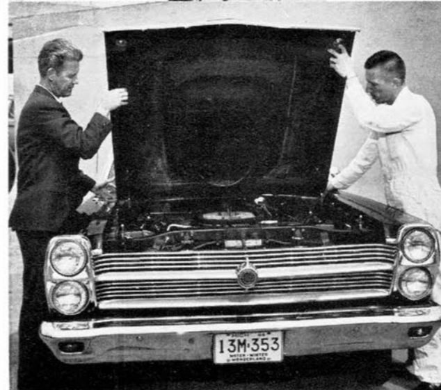
Bill Holbrook, left, and Rolf show filter pack and air cleaner top can be removed to receive direct shot of atmosphere blasting through functional hood scoop.
