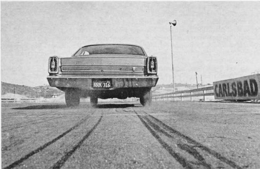
WHEELSPIN POSES something of a problem on acceleration runs. Super Sport tires are good, but drag slicks would be a vital improvement.
