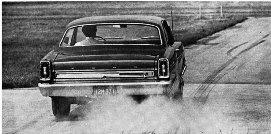
Tire-searing starts in either first or second gear are possible with extra power available. Torque-converter drive allows easy control of wheelspin for fast starts.
