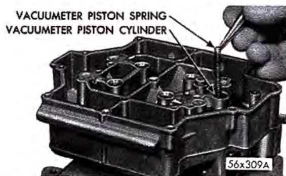
Fig. 36 - Installing Vacuumeter Piston Spring
