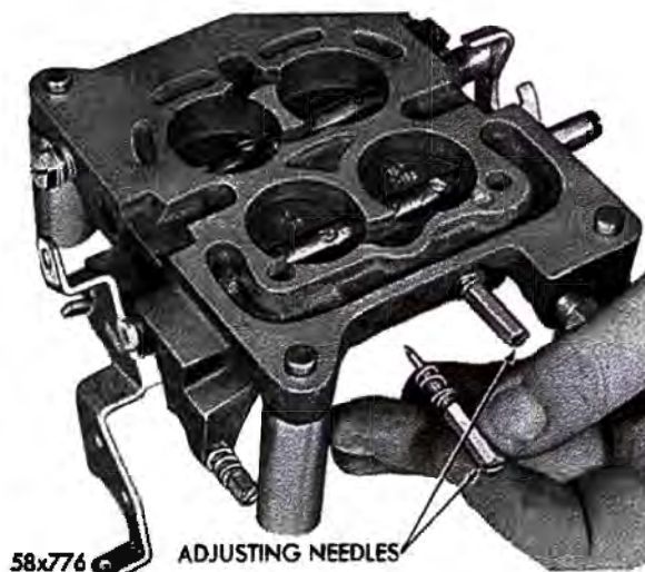
Fig. 28 - Removing or Installing Idle Mixture Adjusting Needles
