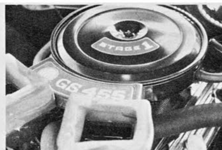
Rubber takes care of sealing the unusual plenum-scoop fresh air arrangement.
