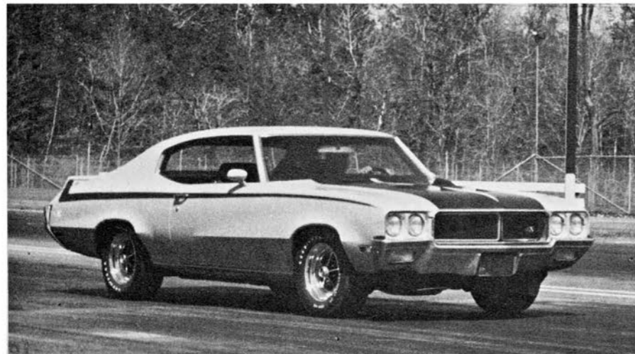
Above, the GSX handles well on both road course and drag strip. Right, the 455-incher takes care of movin' 3988 pounds—right on!
