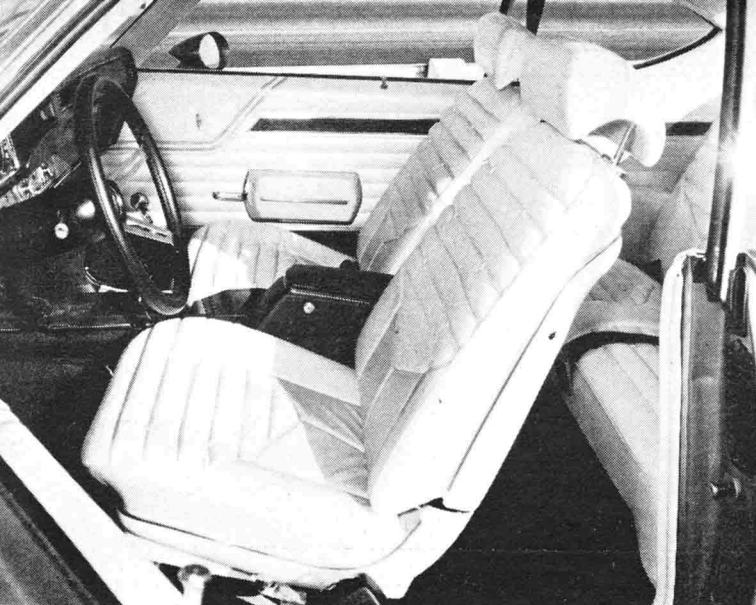
STRATO buckets were wide and raked. Minimum leg room plus low rear window made back fit only for jockeys and kids.
