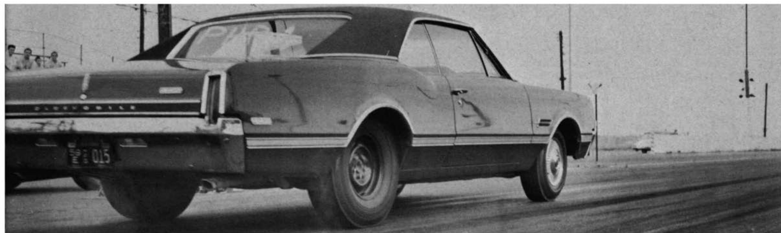
The anti-spin rear-end kept traction on both tires equal. Here car is using a set of slicks for bite.
