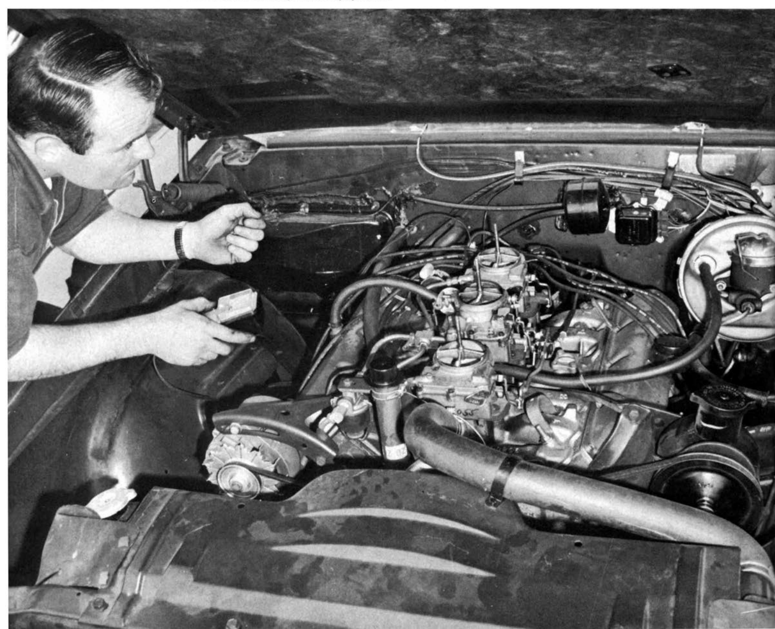
Timing and dwell was checked by Dan Horan, who drives the Allen Paul Oldsmobile 4-4-2. Best timing was slightly advanced from stock setting. Three carbs are of Rochester make and listed as optional equipment.
