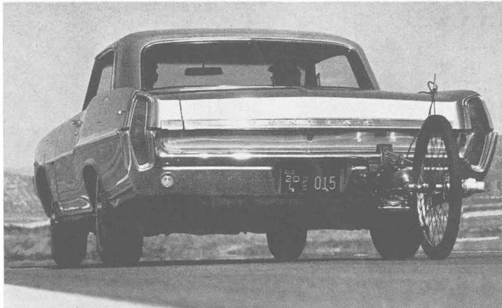
Cool one comes off line without wheelspin. Mileage ranged from high of 14.2 to low of 7.9 mpg, with overall average at 11.8 mpg. Pontiac has more economical V-8 option.
