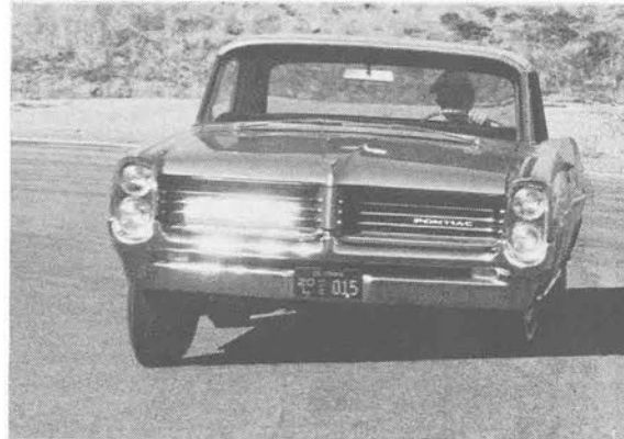
Cool one understeered and scrubbed front tires when pushed hard through fast turns.
