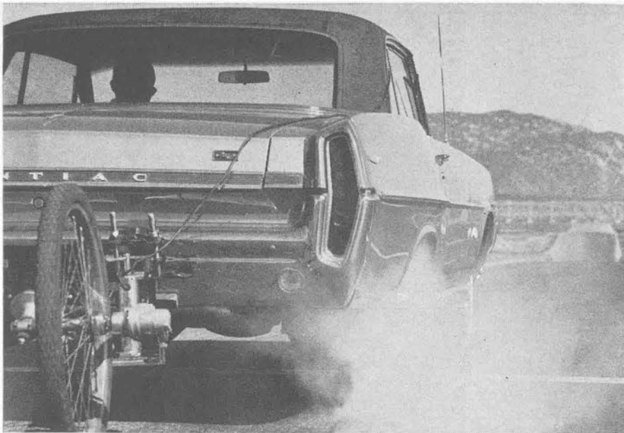
After 1300 miles, most of them fast, the 2 + 2 averaged 10.9 mpg, with a high of 12.8 and a low of 7.1 mpg. Traction was hot car's biggest problem during acceleration runs.
