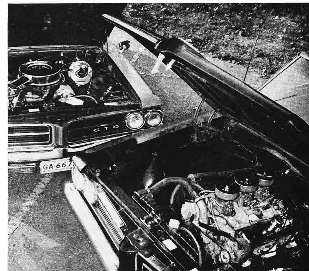
Single quad engine is rated at 325 hp, while tri-power version grinds out 348 hp.
