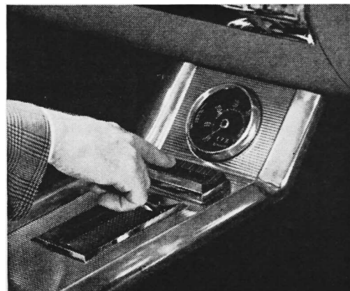
A tachometer shows engine rpm's to tell you when you approach or pass peak performance efficiency.
