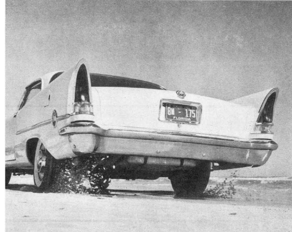
CHURNING THE DIRT will hold any good accelerator back, but on pavement the 300-C does 0-60 mph in 7.7 seconds with the standard rear axle ratio. Other gearing is optional.
