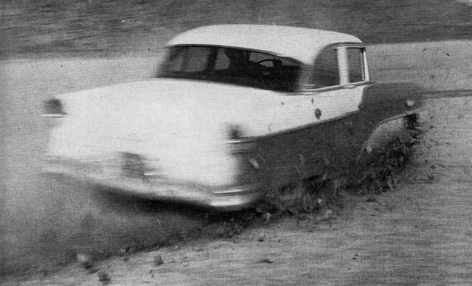
Clipper hits a sharp corner hard. Although wheels dig in deep, the body holds an even keel—a benefit from new torsion bars.
