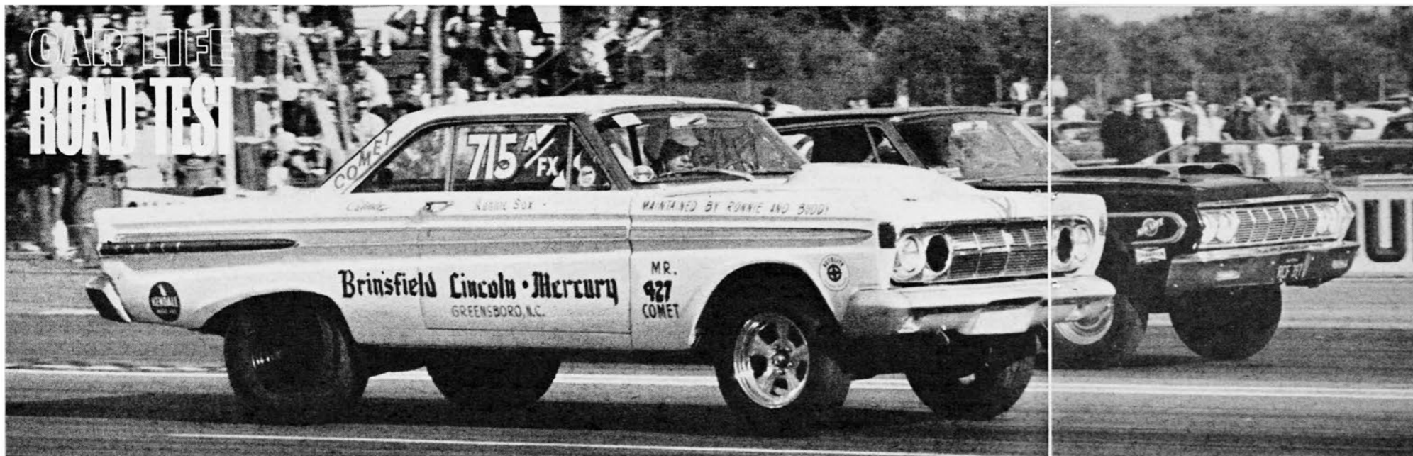
COMET IN action shows stability of the package despite the torque of the 427-cu. in. V-8 and the 4.56:1 gear ratio. This Comet A/FX, driven by Ronnie Sox, is identical to the Chrisman-Shrewsberry car.
