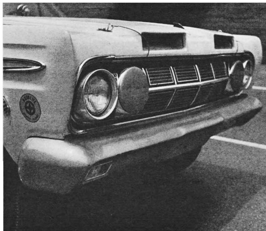
RESTYLED HOOD scoops have increased performance of the dragstrip Comet, evidently by providing a better airflow to the dual Holley carburetors. Bumper is fiberglass.
