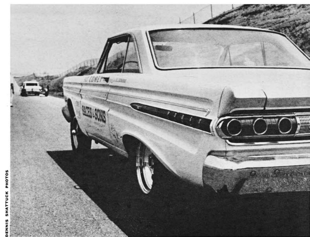
READY FOR a charge down the dragstrip, the Chrisman-Shrewsberry Comet has a power loading of 8.06 lb./bhp. Back window is glass, others are light plastic.
