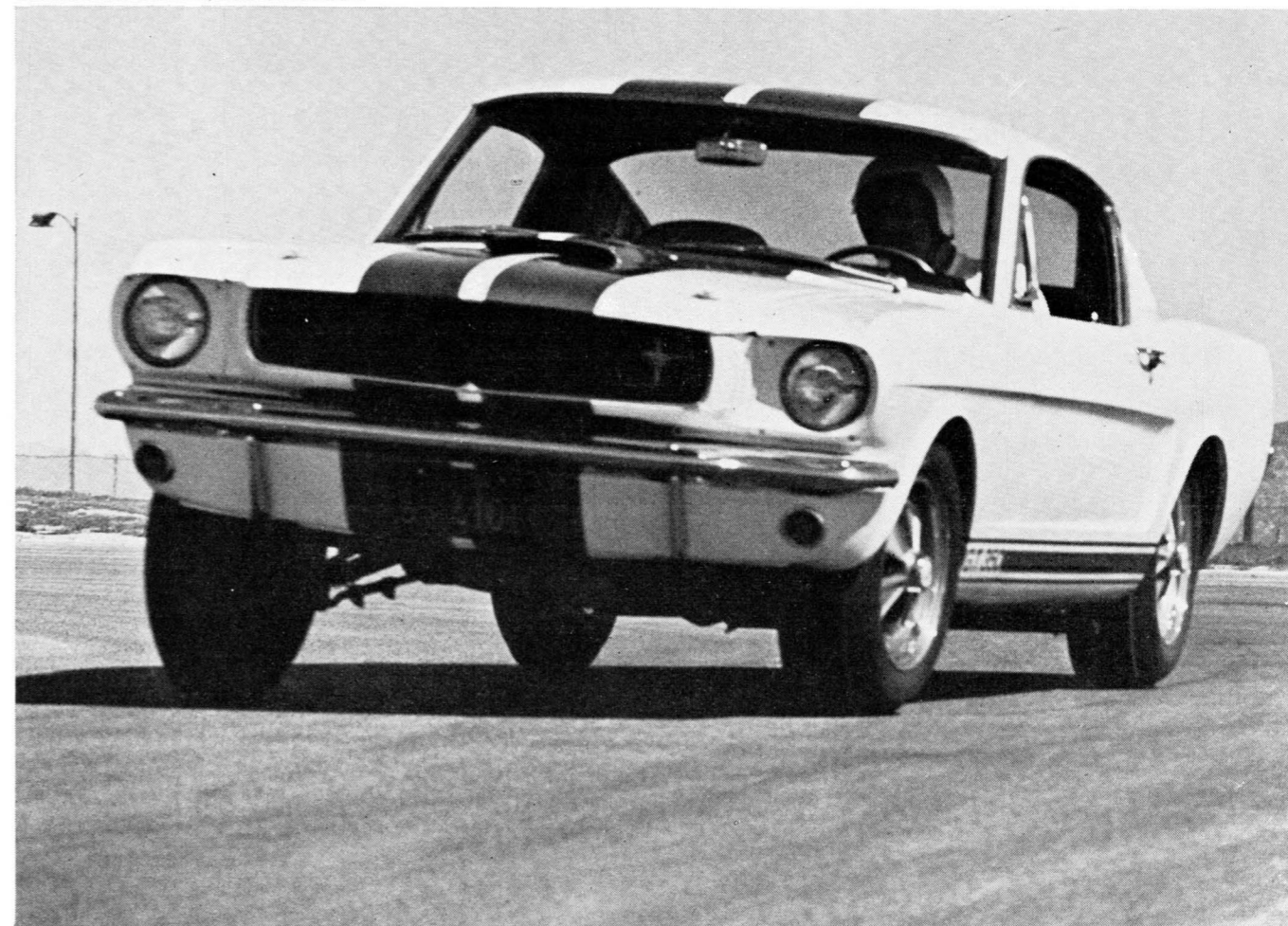
AT NEAR MAXIMUM CORNERING CONDITIONS, THERE'S VERY LITTLE LEAN. BLUE SPOT TIRES STICK AND DON'T ROLL UNDER LIKE ORDINARY ONES.
