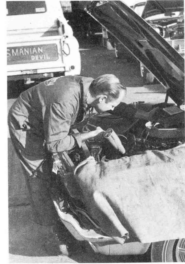
Charlie Dodge and George Snizek tuned both local test cars at their well-equipped speed shop. George, left, points out a trouble spot under the Barracuda hood. Fuel filter and steel lines conducts heat and cause percolation and vapor lock. Charlie, below, puts the timing light on the potent 271 hp mill. Both engines run large single quad carbs.
