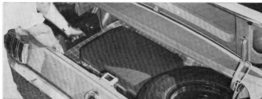
Spare takes up most of trunk space, but there was room for attache and companion cases plus some soft luggage. Lip is high; trunk has lots of sharp edges that could cut.
