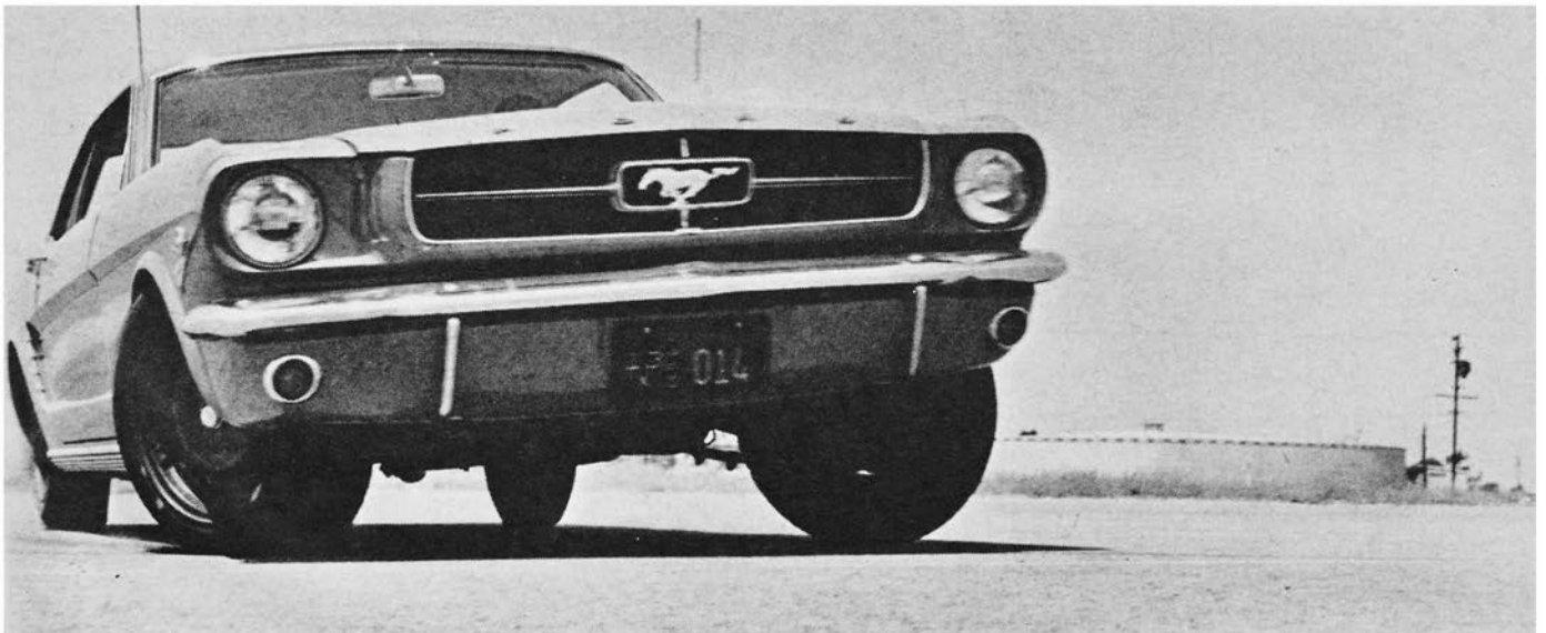
TIGHT CORNERING still produces some body lean, but considerably less than experienced with standard suspension. Rear springs are stiffened more than fronts, but larger anti-roll bar keeps things under control.
