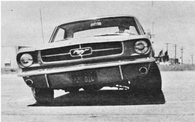
TIGHT CORNERING still produces some body lean, but considerably less than experienced with standard suspension. Rear springs are stiffened more than fronts, but larger anti-roll bar keeps things under control.
