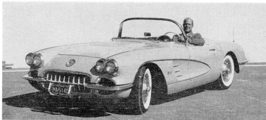
The '58 Corvette has been given a drastic face-lift while still using the same basic body shell. Quad headlights are standard equipment and only the 283-inch V8 engine is available, but with fuel injection and Duntov camshaft, rating is at 290 horses.
