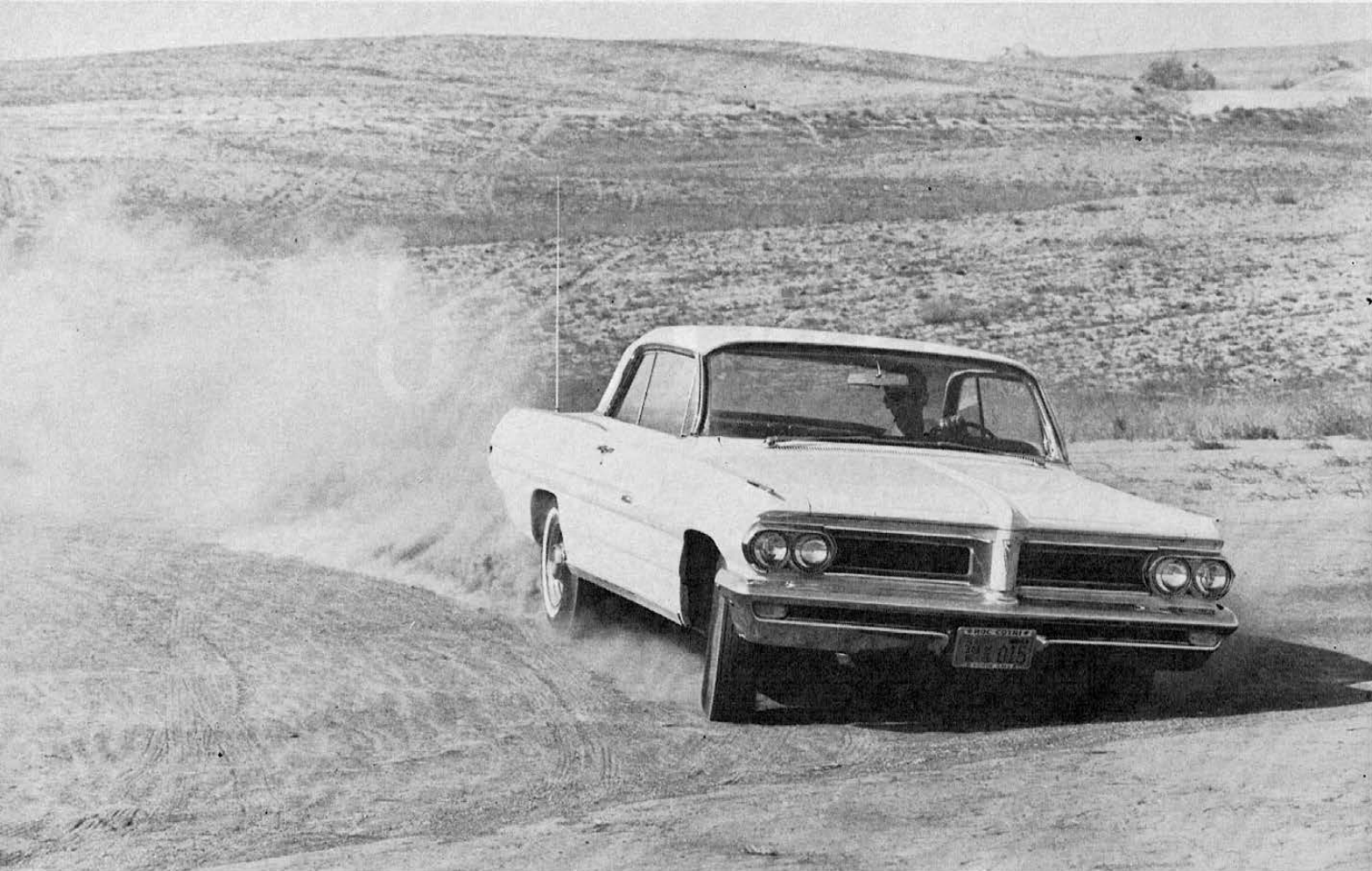
THE GRAND PRIX HANDLES WELL ON ROUGH, LOOSE SURFACES BUT COULD BE GREATLY IMPROVED WITH STIFFER SPRINGS AND BIGGER SHOCKS.
