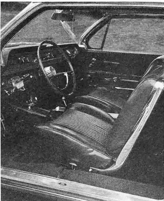
INTERIOR of Grand Prix features bucket seats. SHIFT LEVER is mounted in console. BIG, 421-CU. IN. engine is offered with up to 432 bhp.
