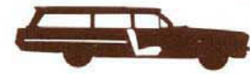
Catalina 6-passenger and Bonneville Custom Safaris —With second seat folded—3 passengers . . . over 8 feet of load length or 36.2 sq. ft. of floor area (tailgate closed). Allowable load plus driver—1,050 lbs. Open tailgate adds over 2 feet of load space.
