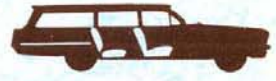
Catalina 6-passenger and Bonneville Custom Safaris —With both seats up—6 passengers plus 300 lbs. of cargo . . . 5 feet of load length or 18.5 sq. ft. of floor area (tailgate closed). Allowable load with driver—1,050 lbs. Open tailgate adds over 2 feet of load space.
