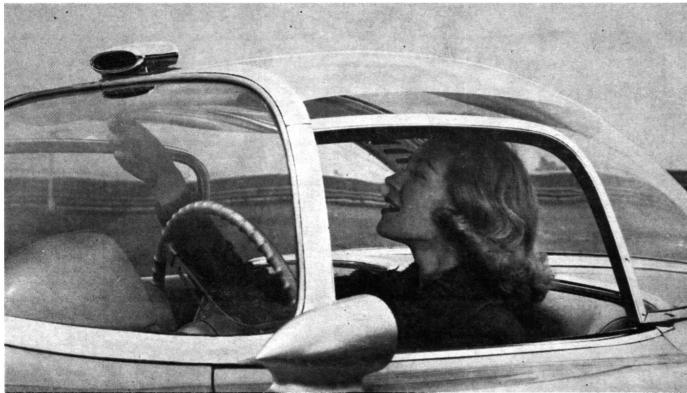
Pretty model adjusts periscope rear-view mirror in bubble canopy. It gives clear view of road behind.
