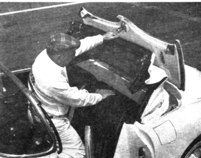
Well-fitting hatch covers storage space for heavy-duty canvas top that can be raised or lowered quickly by one person without tools. Roll-up windows fit snugly.
