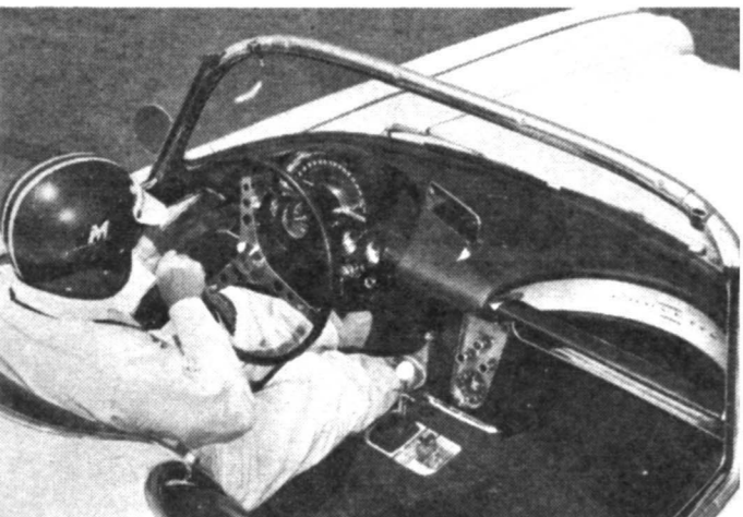
Racing-type cockpit, with 3-spoked wheel, short-stroke, positive manual shift, and individual bucket-type seats, is functional for racing, comfortable for road touring.
