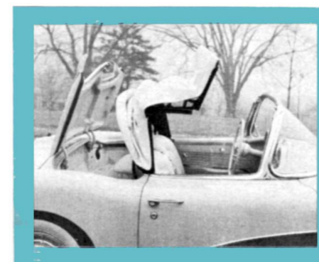
Fully automatic, the top slips out of the well after the lid raises. Convenience of automation makes added weight of unit bearable.
