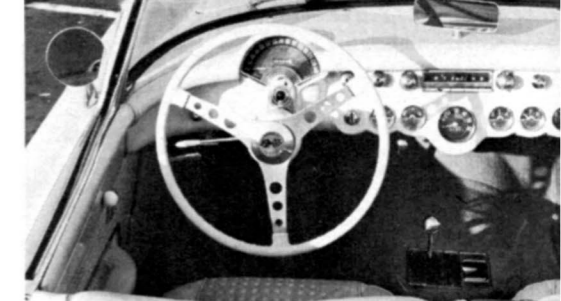
Instruments are well balanced for eye-appeal, but not practical. Reading them at any speed over forty is difficult. Note simple design of steering wheel.
