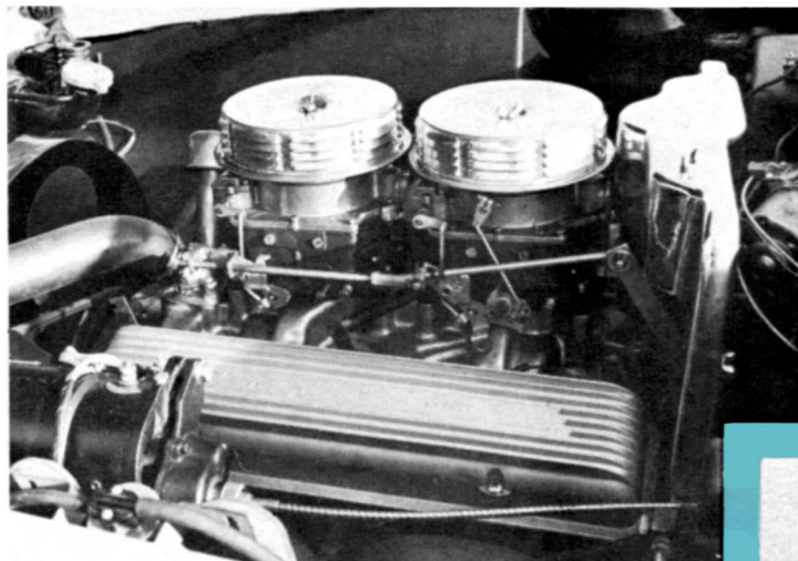
Twin four-barrel carburetors squat on power plant ready to help deliver 225 bhp at 5200 rpm. At low speeds, only rear carburetor functions. BELOW —Hood raises from rear, reducing possible lifting at high speed. Engine compartment is more accessible for shop work.
