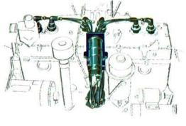
Safeguards engine by removing dirt and other harmful abrasive particles from the engine oil. Every drop of the oil is
