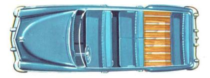
The wide front and rear seats will comfortably accommodate six passengers. Either, or both sections of the rear seat can be folded forward for more storage space. Removable seat in rear compartment for children is optional equipment.
