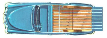
The tailgate lowers flush with the floor for easy loading or unloading. Storage space is 47 inches wide; 35 inches high; and 75 inches long. With rear seat folded forward, and tailgate lowered, storage space is 116 inches in length.
