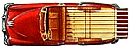
Either half of divided rear seat, or both, can be folded forward to form flat storage compartment 116 inches long.
