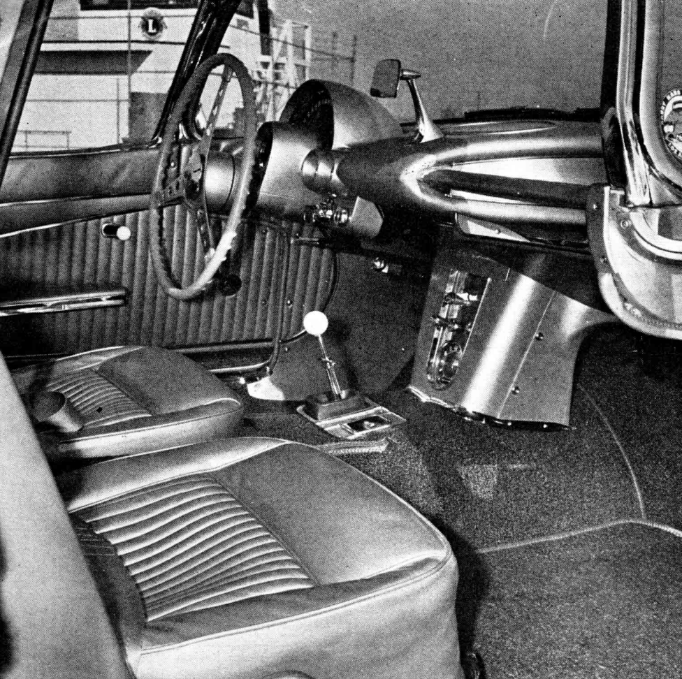
Corvette interior is beautifully styled and well-fitted. Seat belts are standard and each of the bucket seats is adjustable. Steering wheel is nearly vertical and feels awkward at first. Shift lever for the 4-speed is conveniently placed.
