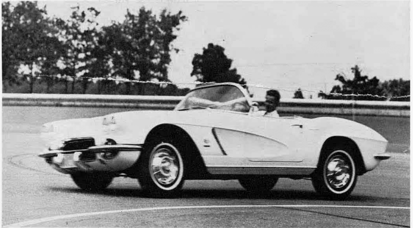
Even though body-roll is moderate in the above photo, we discovered later that anti-sway bar up front had broken. Charts below indicate the wide range of options that enable Corvette buyers to order up anything from "streeter" to race cars.
