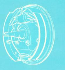
Air-Cooled Brakes for Safe, Positive Stopping! Durable, husky brakes are a vital part of sports car driving—and the Corvette's got the brakes to do the job! New slotted wheel discs permit air to cool the innermost areas of the big 11-inch hydraulic brakes, help maintain constant high-brake efficiency and add extra lining life. Brakes are self-energizing with faderesistant, bonded linings.
