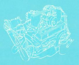
Power with the Sweet Sound of Action! The life blood of Corvette performance comes from its Chevrolet-engineered 283-cubic-inch (4.7 litre) Corvette V8! You get this V8 in five great Corvette versions . . . ranging from the standard 230-h.p. V8 with 4-barrel carburetion to the 290-h.p. Corvette V8\* with Ramjet Fuel Injection, attaining over one h.p. per cubic inch of displacement . . . a dramatic achievement for American production engines!
